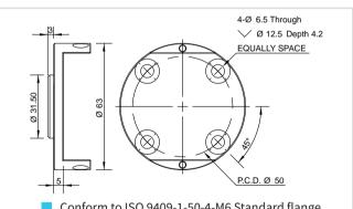
Conform to ISO 9409-1-50-4-M6 Standard flange \*If you need to customize the flange, it is recommended to design according to the robot installation hole position, or contact us
